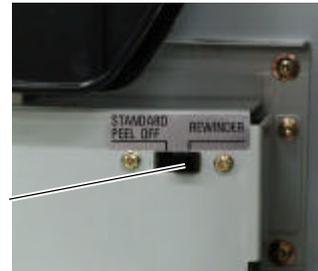
2. The backing paper can be wound directly onto the Take-up Spool or a paper core.
