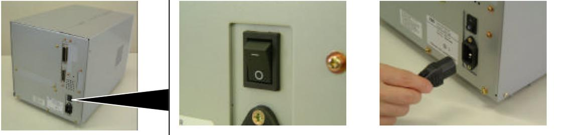
2. Never perform disassembling, assembling, and cleaning just after printing. Doing so may cause you to be injured by the print head and the inner parts of the printer being hot.
