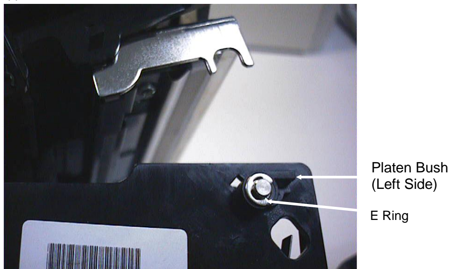
Remove E ring and platen bush
