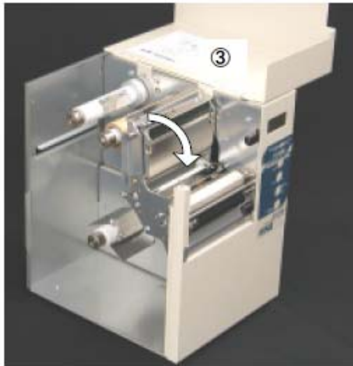
Fig.3.2c When the print mechanisms is open with maximum angle.
